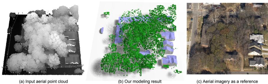
**Fig. 1.** Given (a) a dense aerial LiDAR scan of a residential area (point intensities represent heights), we reconstruct (b) 3D geometry for buildings and trees respectively. (c) Aerial imagery is shown as a reference.
