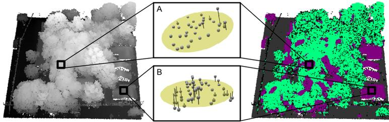
**Fig. 2.** Local geometry features become unreliable when dealing with residential areas with rich vegetation. In closeups of (A) a tree crown region and (B) a rooftop region, points are rendered as spheres while a locally fitted plane is rendered in yellow. Right: classification results of [18], trees in green, buildings in purple, and ground in dark grey.
